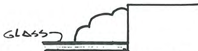
GLAZING STOP - INTERIOR THIS MOULDING IS IN FOUR PARTS AND CUT TO FOLLOW THE ELLIPTICAL GLASS SHAPE
