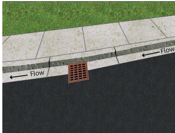
Figure 6-5 - Single Catchbasin on a Continuous Grade
