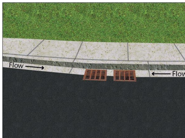
Figure 6-6 - Double Catchbasin in a Sag
