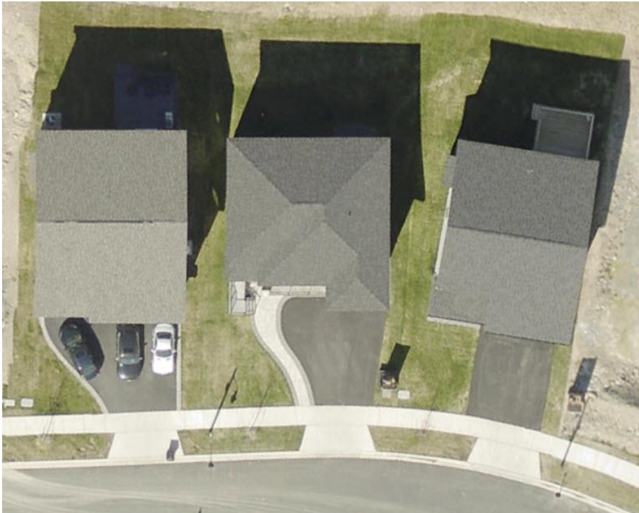
Left: Triangular driveway with reduced snow storage. Center: Triangular driveway widened with an adjacent walkway. Right: Driveway with consistent width but installed wider than approved.
